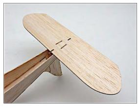
Fit/glue lower fin V4 to horizontal stabilizer and V2. Double the fake tailwheel/skid with two V5 1/32 in. ply disks.
