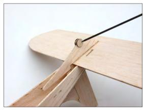
Bend landing gear per plan sheet and fit to gear block.
