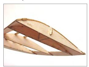
Sight along flats of ribs forward of spar S3 to ensure wings are not warped. If you discover that your wings are warped: Lightly mist wing with glass cleaner solution and pin to a flat work surface. Allow to dry completely before removing. Lightly sand wings to a smooth finish.
