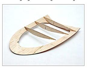
tape the leading edge to the work surface, then wrap the frame over the ribs and glue at trailing edge.
