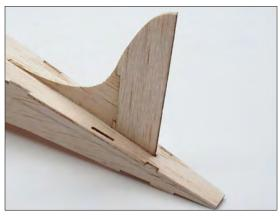
Fit horizontal stabilizer H1 to bottom of fuselage using tabs on fuselage and bottom of vertical stabilizer to align. Square stabilizer to vertical fin and glue.
