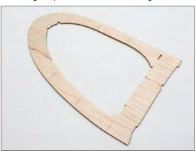
Fit and glue rib R2 to slot in leading edge of wing.
