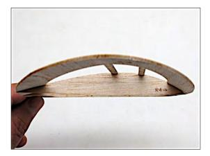
Cover model using small swatches of light weight covering material such as AeroLite. Cover only the TOP surface of the wing. Performance of this model will be reduced SIGNIFICANTLY by covering the underside of the wing.
