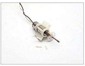
Install motor so shaft points slightly to the right of the aircraft centerline. Secure with medium CA.
